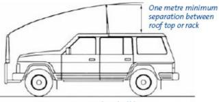
Antenna mounted on bull bar
