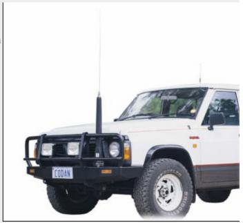
The main antenna section is constructed of fiberglass reinforced nylon. This provides a weatherproof housin for the control and tuning devices, which are fitted inside. It is mounted on an anti-vibration base that incorporates rubber mounts. These are likely to be met while travelling on unsealed roads or tracks.
