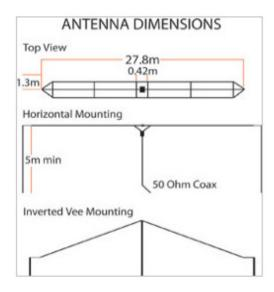
BBA-1000 Broadband multi wire base antenna for 1 Kilowatt PEP. Sturdy Stainless steel and fibreglass construction, can be mounted horizontally or as inverted V. Supplied with 30m of coaxial cable and instructions.
