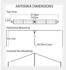
BBA-500 HF Broadband multi wire base antenna. 500 Watts PEP. Sturdy Stainless steel and fibreglass construction, can be mounted horizontally or as inverted V. Supplied with 30m of coaxial cable and instructions.
