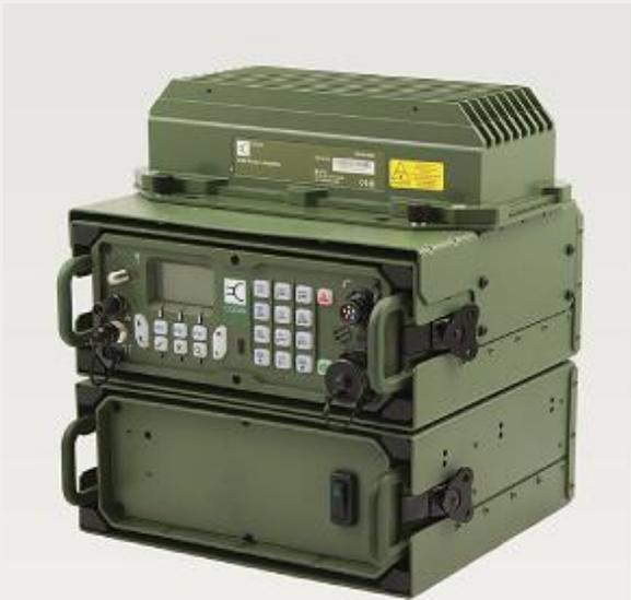
The 2110M-B125 is a compact 125 watt base station system utilising the 2110M manpack radio and the 3160 125 watt power amplifier. Coupled with Codan's 3520 power supply, the system is operational from DC and AC mains supplies, auto switching to DC with loss of AC.
