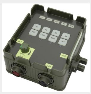
The Basic Crew Unit (BCU) is a simplified, easy-to-use, crew station for direct internal communication and for using the radios in the vehicle as authorized by the Commander (using ACU). Like the ACU, this BCU module also contains a DSP that controls its functions, and features Dynamic Noise Reduction and VOX activation for clear, reliable communication.
