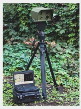
The complex is a multifunctional optoelectronic device designed for twentyfourseven video monitoring of the terrair aims searching and automatic detection of camouflaged optical aiming and tracking devices, determination of their coordinates and distance in difficult terrain and urban buildings conditions.
